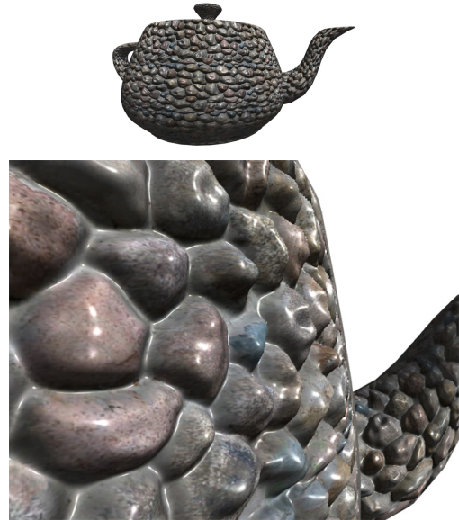
Figure 16: Relief texture-mapped teapot (top). Close-up view produced with a 512x512 stone relief texture (bottom).
