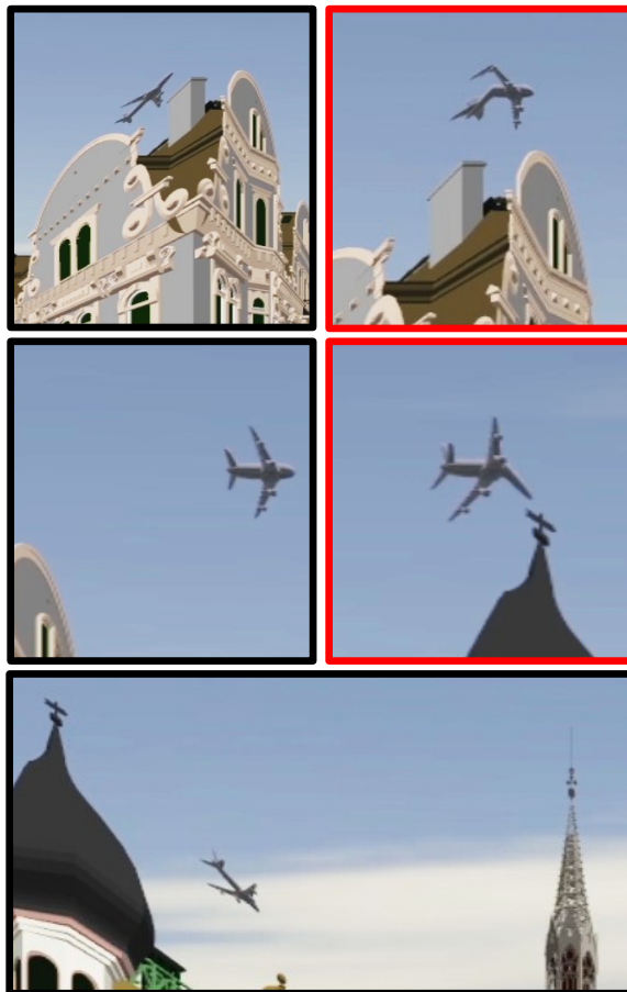
Fig. 11. Fragments of the multiperspective visualization from Fig. 9 showing an airplane flying overt the buildings. The airplane appears distorted as it crosses from one camera segment to the next (images with red border) and it is not distorted while completely contained by one segment (images with black border).
