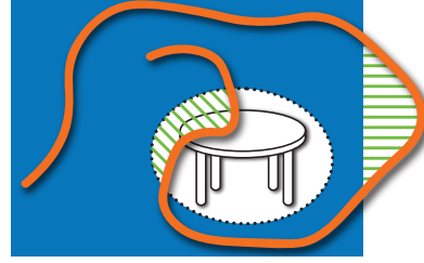
Fig. 5. Error measure for user studies. We compute the error \epsilon in Equation (9) as the total area (shown striped) that is out of bounds or within obstacles.
