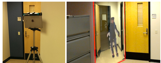
Fig. 3: Left: the RGB camera with depth sensor accessory captures a RGBD video stream that is converted to a 3D point cloud. Right: the point cloud, as seen from the secondary perspective, is integrated into the primary perspective in the multiperspersive visualization.
