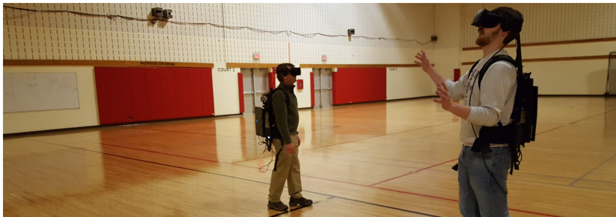
Fig. 1. Two immersed users are redirected around each other as they explore a virtual environment.
