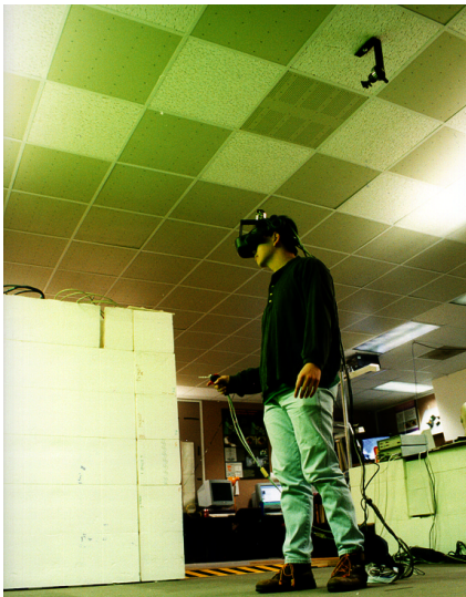
Figure 7: A user wearing the HMD and the wide area tracker
