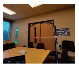
Figure 3: Frame captured from the learner's XR headset. The learner uses the virtual laser pointer (blue) to probe the firing value of neuron "6" of the SoftMax layer. The value is 1.0, indicating the correct classification of the input image (see Figure 1).
