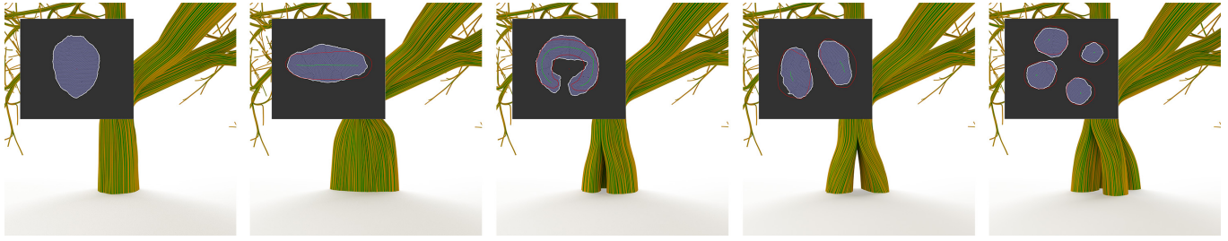
Fig. 12. Branch profile sketches: our method enables users to sketch branch profiles for any node in a branch graph. Possible profiles range from single branches and branches with cavities to split branches.
