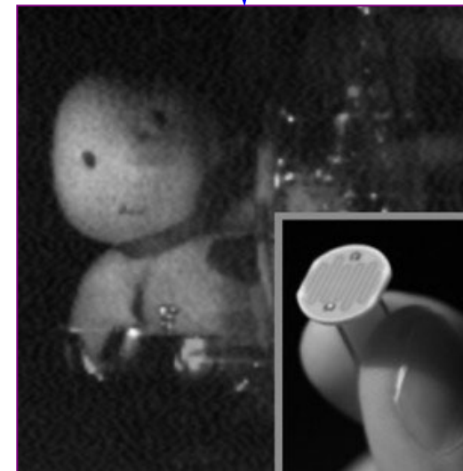
dual photograph, as seen from projector's position and as illuminated from photocell's position
