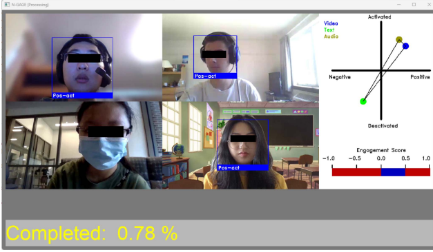
Fig. 9. N-GAGE (Processing) software incorporates the detection of engagement from three separate data streams (video, audio, and text). The detected engagements are displayed on the Russell diagram in real time for each frame of data. Blue, yellow, and green dots denote the predicted engagements from video, audio, and text streams, respectively. The “engagement score” bar denotes the level of team engagement for each frame of the video based on the predictions of the three engagement detectors, with scores of 1, 0.5, -0.5 , and -1 for productive engagement , idle , disengagement , and unproductive engagement , respectively.
