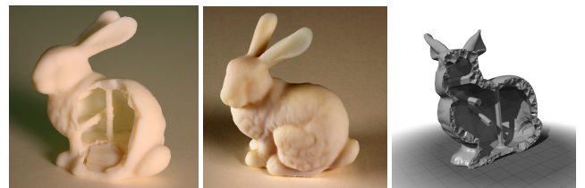
Figure 15: Example of hollowing. A hole is created in the object to save material and to lighten the whole object. Inner struts are added to maintain structural strength.
