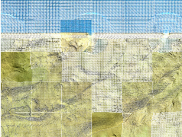
Fig. 4: Each tile covers the same area of the virtual terrain, but its actual resolution depends on the complexity of the underlying layers.
