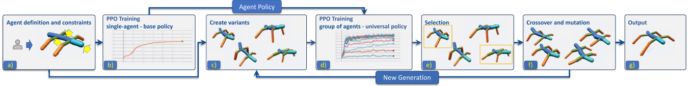
Fig. 2. Overview: The input agent is either generated randomly or by the user, and the user can also define constraints (yellow arrows) (a). The initial Proximal Policy Optimization (PPO) trains the input agent to provide baseline agent policy (b). The algorithm then creates variants of the initial model (c) and trains them with the universal PPO (d). Selection (e), crossover, and mutation (f) create a new generation trained again. The system outputs the best(s) co-designed agents and their policies (g).
