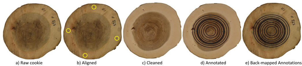
Fig. 2. Overall process pipeline. The raw cookie (a) is marked with drilled holes (shown schematically as circles) for alignment (b) and then cleaned (c). Two images (one from each side) are then taken and the images are manually annotated (d). The annotations are mapped back to the raw cookie and used to train our deep neural network model.
