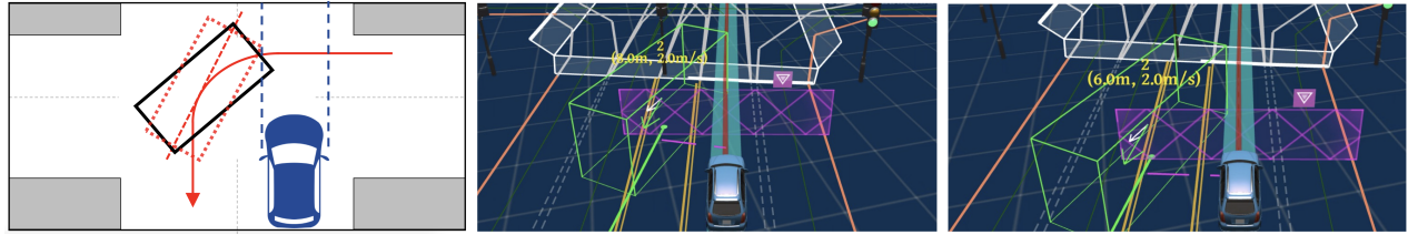
(a) Illustration. (b) Path.theta.v = 10 km/h . Collision. (c) Obs.theta.v = 0 km/h . No collision. Figure 12: Replay Accident A6. In Figure 12a, black box is the truck. Red dotted box is what AD vehicle thinks.
