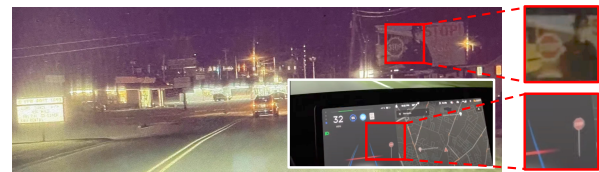
Figure 1: A real-world emergency braking case reported by [7], as the Tesla autopilot recognizes the stop sign from the road-side billboard. Billboards are common and benign, but such scenarios can be accident-inducing.
