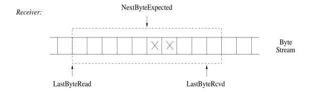
• sender, receiver maintain buffers MaxSendBuffer, MaxRcvBuffer
