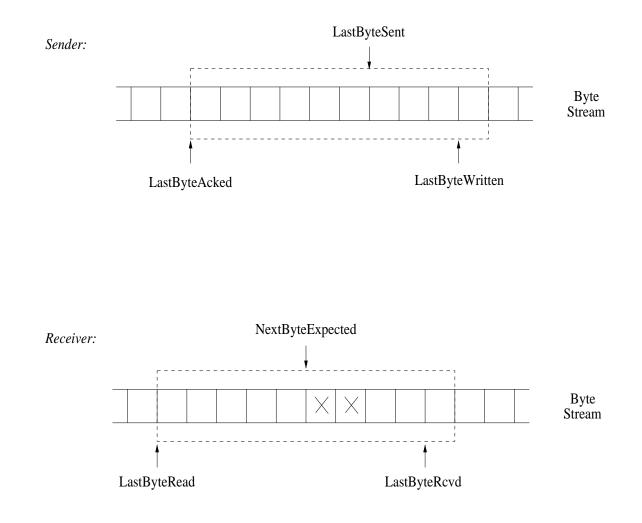
• sender, receiver maintain buffers MaxSendBuffer, MaxRcvBuffer Note asynchrony between TCP module and application.
