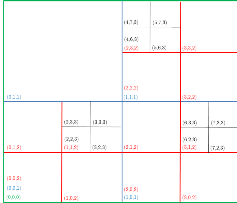
Figure 7.3. An initial grid cell (green) with adaptive cell subdivision applied to demonstrate the associated changes in cell index.
