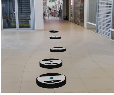
Fig. 5: Moving virtual object, i.e., a robot vacuum cleaner, integrated into the real-world scene. The robot is shown here at several time steps to illustrate its trajectory with a single image.
