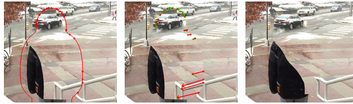
Fig. 7. Local mapping need (left), implementation (middle), and result (right). Left: disoccluding using only the global mapping results in discontinuities where near objects cross the occluder contour, e.g. where the sidewalk and handrail cross the red line in the left image. Middle: the local mapping connects primary frame salient contour points (red points) to their correspondence in the secondary frame (green points); the local alignment offset is larger for near objects. Right: disocclusion with continuity at occluder contour.
