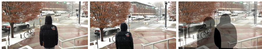
Fig. 5. Initialization of rotation from the first frame of the secondary video V_2^0 (left) to the first frame of the primary video V_1^0 (middle). The rotation is visualized by blending V_1^0 with the rotated V_2^0 (right). The rotation is recovered robustly (see alignment of distant parts of the scene), despite the considerable disparity between the two frames (see ghosting of near parts of the scene).
