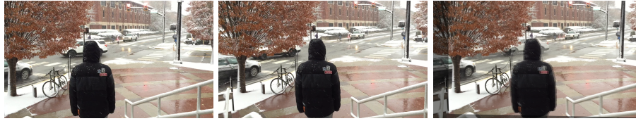
Fig. 6. Global alignment of two primary video frames (left and middle). The frames differ in view direction (see light post), and in time (see turning car). The blended visualization (right) shows that the global alignment recovers the rotation robustly (see alignment of distant scene), despite the motion in the scene (e.g., turning car) and the disparity of near objects (e.g., occluder and handrail).
