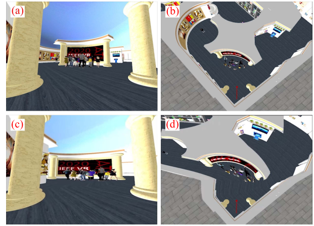
Fig. 11: Illustration of the VE warping induced by our multiperspective visualization: (a) conventional user view, (b) third person view of original VE, (c) multiperspective visualization, and (d) third person view of warped VE, which, when rendered conventionally, produces image (c).
