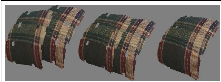
Figure 10 Depth then color registration: pair of frames before depth registration ( left ), after depth registration ( middle ), and after color registration ( right ).
